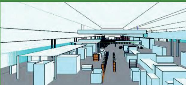
The 3D RF propagation simulations of the 20,000 square metre Smart Factory provided significant advantages when determining the number of base stations required, the preferred locations and the appropriate antenna tilt, with proper attention paid to vital restrictions on where the base stations could be installed.
